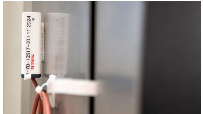
A mini data logger in use for a Thommen Medical heating cabinet: For optimum use, the sensor inside was connected to the data logger using a ribbon cable.
