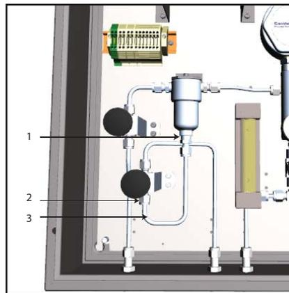
3. Disconnect the tube with its fitting (3).
