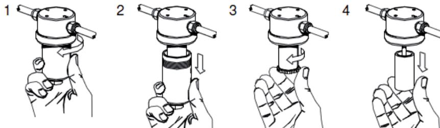
Remove the bowl (1,2), element retainer (3) and filter element (4).
