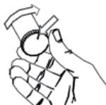
The filter tube is securely sealed by tightening the element retainer a 1/4 to 1 turn after it first contacts the filter element, the amount will depend on the housing type and element size. A mark on the end of the retainer is used as a guide.
