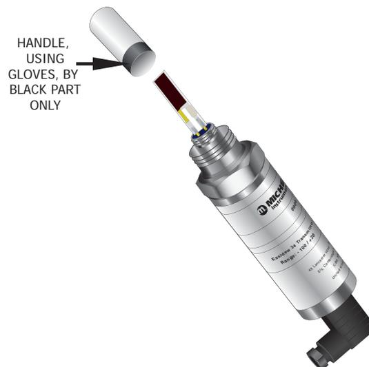
Figure 1 *Replacement of HDPE Guard*
