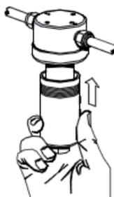
4. Re-connect the tube with its fitting to its original configuration.
