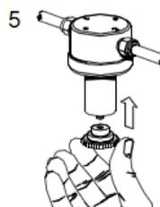
Disposable and sintered PTFE filter elements are sealed by compression against a flat surface (5). Gaskets are not required between the filter element and components of the housing. The element is located by guides which fit the inside diameter of the tube at each end.
